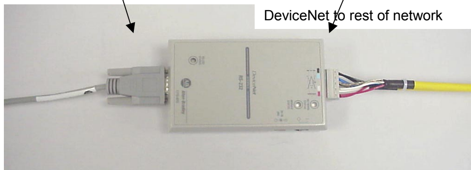
Photo of 1747-KFD serial RS-232 DeviceNet interface
