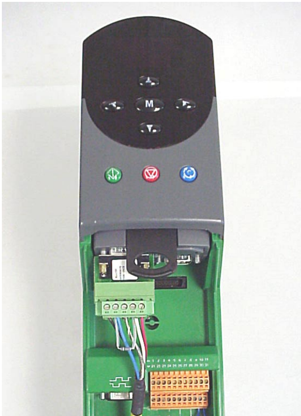
Photo of 121-ohm 0.25 Watt Termination Resistor fitted to UD77 at the end of the Trunk Line (furthest from the Scanner)
