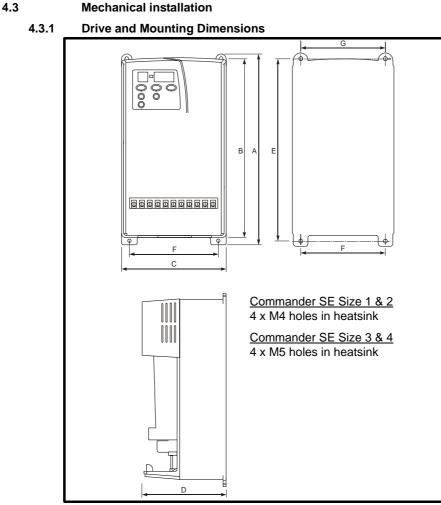
Figure 4.1 Drive and mounting dimensions
