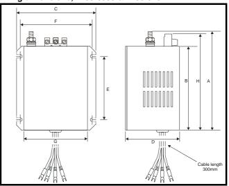
4.3.5 Commander SE Size 2, 3 and 4 Low cost three phase RFI Filter mounting dimensions, 4200-6303 & 4200-6402.
