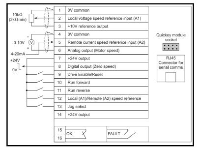
Figure 5.3 Control terminal connections
