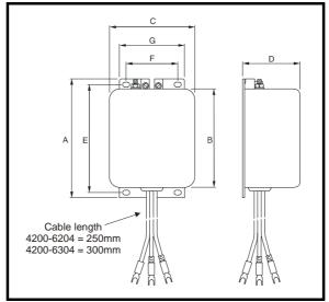
Figure 4.4 RFI filter dimensions
