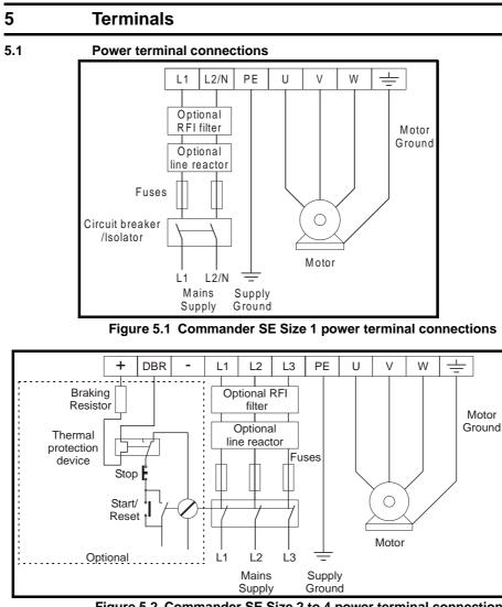
Figure 5.2 Commander SE Size 2 to 4 power terminal connections
