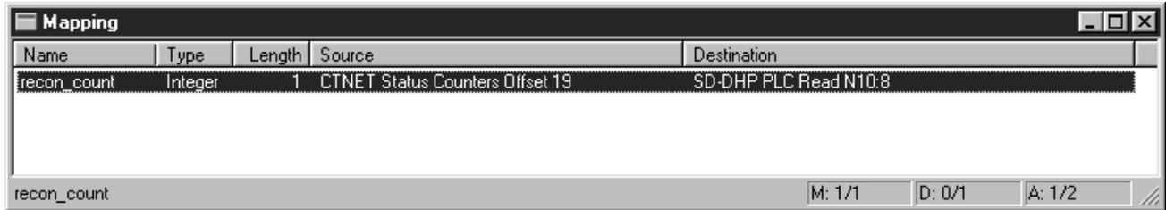
**Figure 41. Mapping the RECON counter to a PLC Register**
